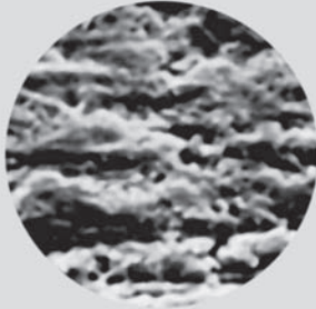
Gel-Coat after sanding – center magnified 1000 times.
