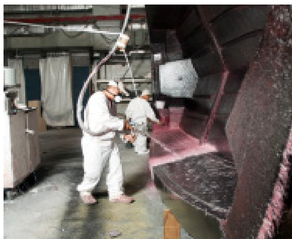
Figure 2 Regal Operators Spraying OptiSpray™ rovings on a Complex Mold.
