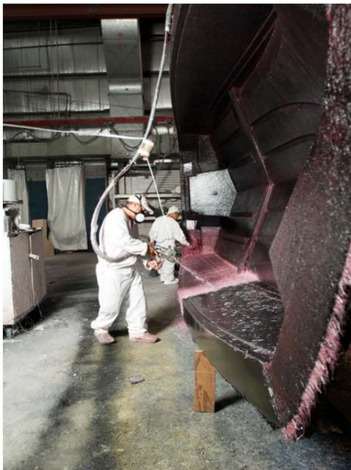
Figure 2 Regal Operators Spraying OptiSpray™ rovings on a Complex Mold.
