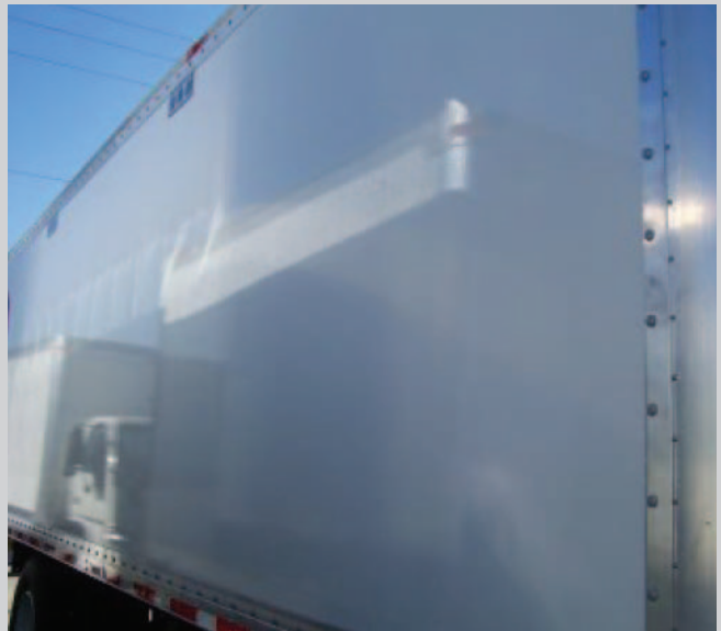
▲ Used in place of through-bolts on truck bodies, adhesives help reduce corrosion and installation time. Photo courtesy of Henkel Technologies.
