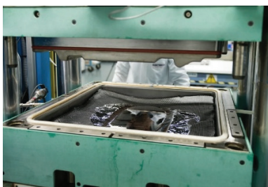
Install wet-out part in mold
