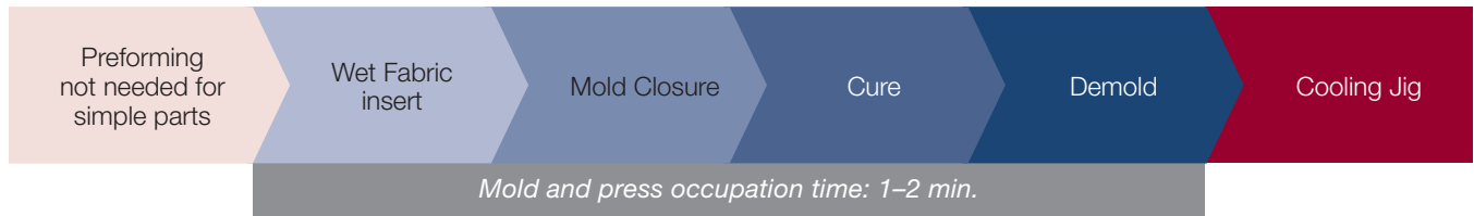
Figure 3. Wet Compression Molding Process
