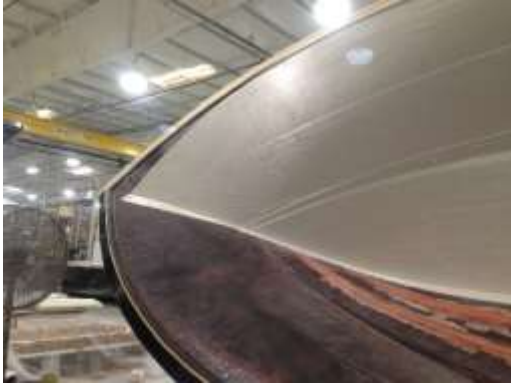
Skin coat is shown at the bottom with the first layer of fabric at the top.
