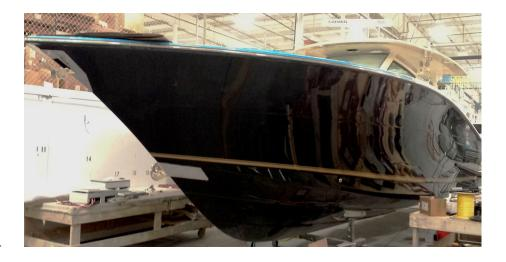
schedule, are put down. Lightweight, rigid foam core is sandwiched between the fiberglass laminate layers. Next, a tackifier adhesive is sprayed over all plies to secure them in place until the epoxy is infused. To optimize the infusion process, a layer peel ply backed with external flow media is put down.
