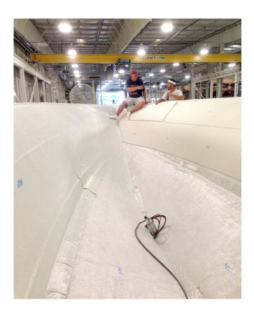
to see. Fabrication with polyester resins often requires the addition of print blockers and barrier plies to prevent surface distortions and imperfections. In addition, completed hulls typically need time-consuming secondary rework and refinishing." The black 420 LXF epoxy-infused hull requires little, if any, secondary finishing after demolding and thereby provides for significantly reduced labor time and faster overall production speed.
